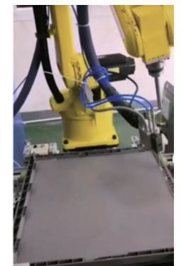
Gluing of control cabinet doors
