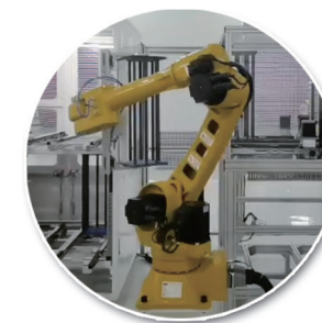
Photovoltaic basket handling
